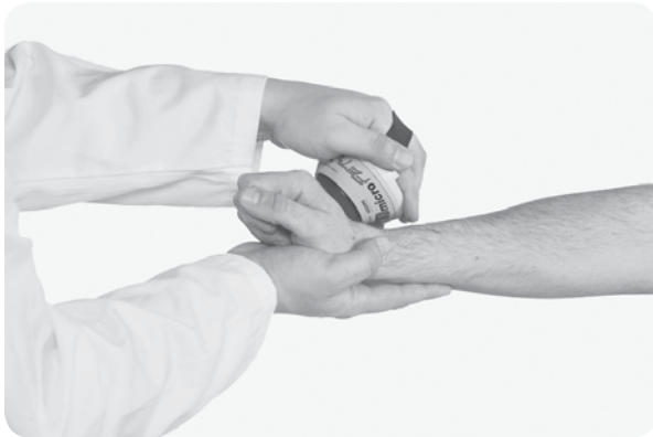
FIGURE 6.4 (a) Handheld dynamometer for measuring isometric strength and (b) the hand being tested.
