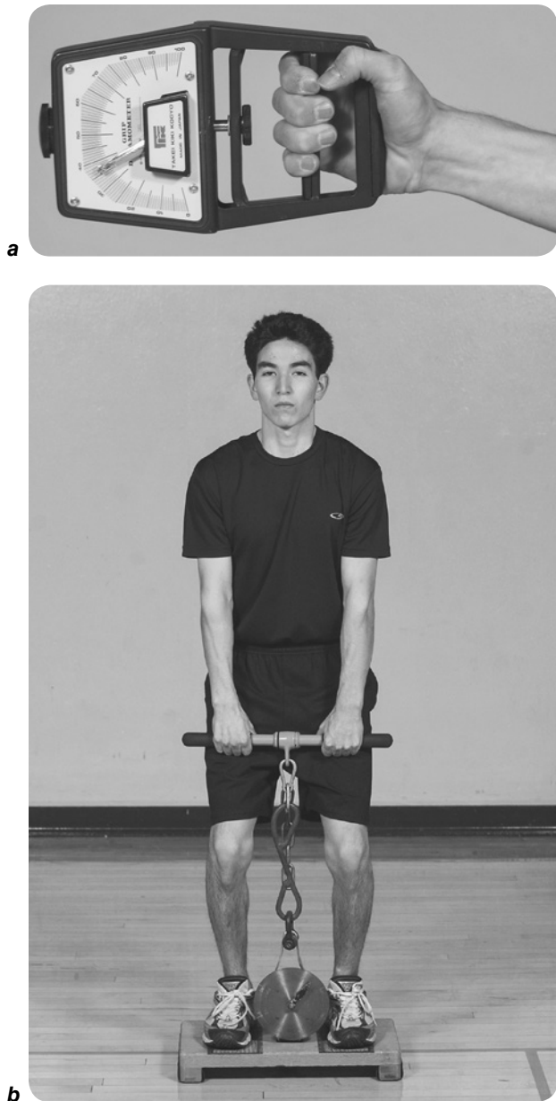
FIGURE 6.3 Spring-loaded dynamometers for measuring static strength and endurance: (a) handgrip dynamometer and (b) back and leg dynamometer.
